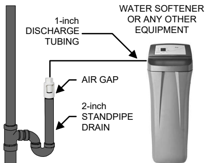
Example of the air gap installed on a 2-inch standpipe.
