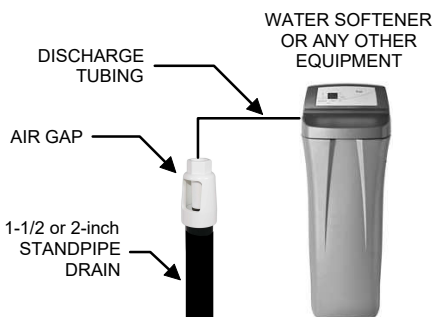
Example of the air gap installed on a 1-1/2-inch standpipe.
