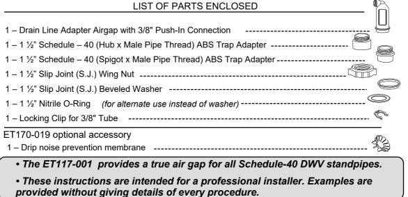
To <u>comply</u> with all plumbing code requirements, the standpipe used with an ET117 series must be trapped, vented and fabricated from a Schedule-40 Drain Waste and Vent that has been approved in your area, such as: ABS, PVC, galvanized steel, copper, or no-hub cast iron with an inside diameter of 1-1/2-inch or greater.
