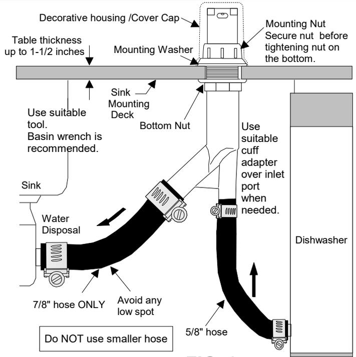
6. Install the decorative cap by pushing it down over the housing to cover the mounting nut and washer. Rotate the decorative cap so the two air gap openings face the sink.
