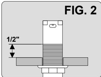
4. Orient the bottom inlet and outlet under the sink as desired. Then, pull down on the air gap while tightening the bottom nut clockwise. **DO NOT OVERTIGHTEN.**
