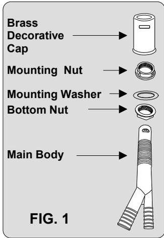
2. Remove decorative cap. Unscrew and remove the mounting nut and mounting washer from the AG300-00X body. Turn the bottom nut counterclockwise further down the air gap's body. Leave sufficient length for the air gap to protrude through the mounting hole. (See Fig. 1)
