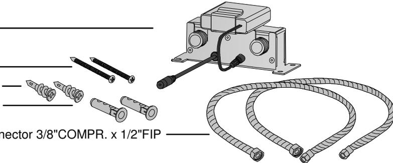
**The AG250-003, in combination with AG250 series foot pedals, provides hands free faucet operation. Pedals are ordered separately. Select from the following three foot pedals: AG250-403, AG250-503 or AG250-603.**
